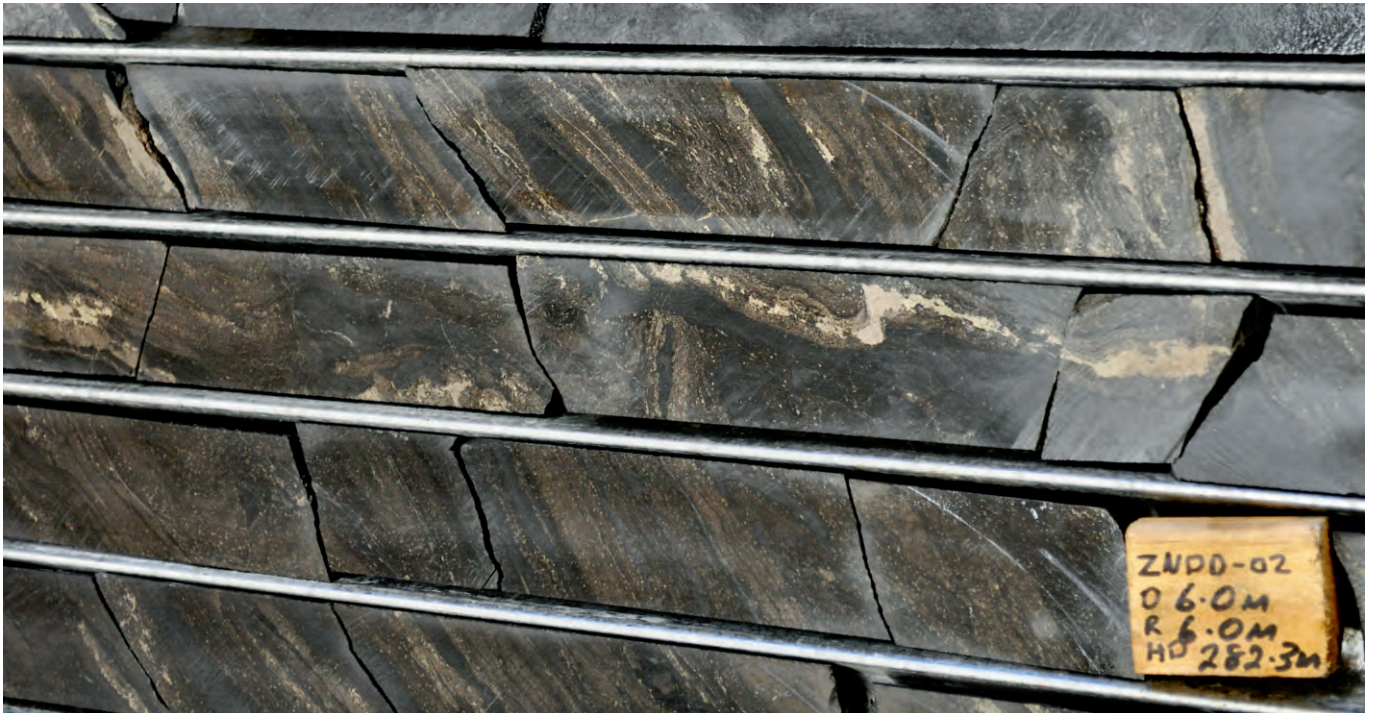
Figure 4.2: Drill core ZNDD02 (top) showing intersected mineralisation and gossan surface expression of mineralisation (bottom) (Heron Resources)
