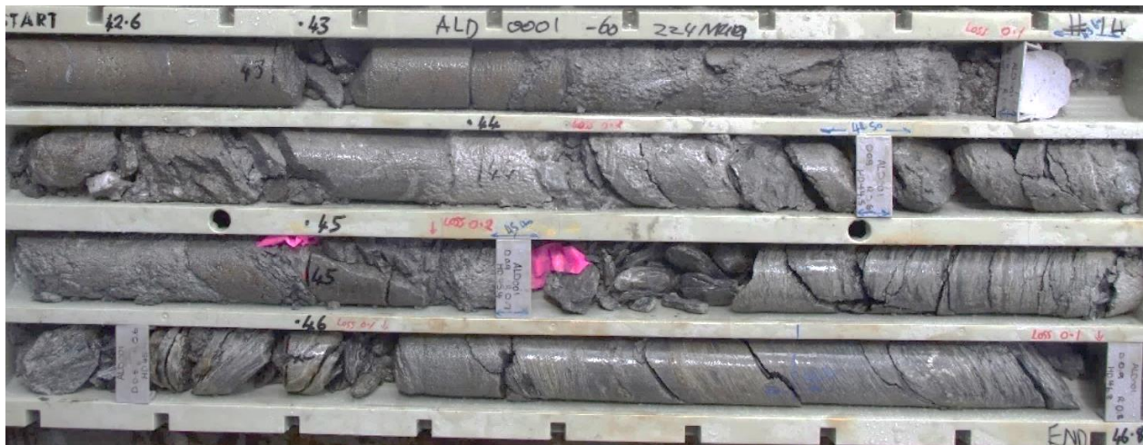
Figure 1 – Mineralisation in ALD0001 (deep bronze colouring) (tray 14, 42.6 to 46.8 m).
