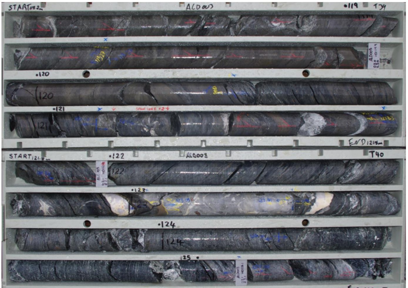
Figure 1 – Mineralisation in ALD0003 (119.27-120.48m, 1.21m at 14.29% Zn equiv), typical intense chlorite-pyrite alteration associated with Stringer Zone mineralisation
