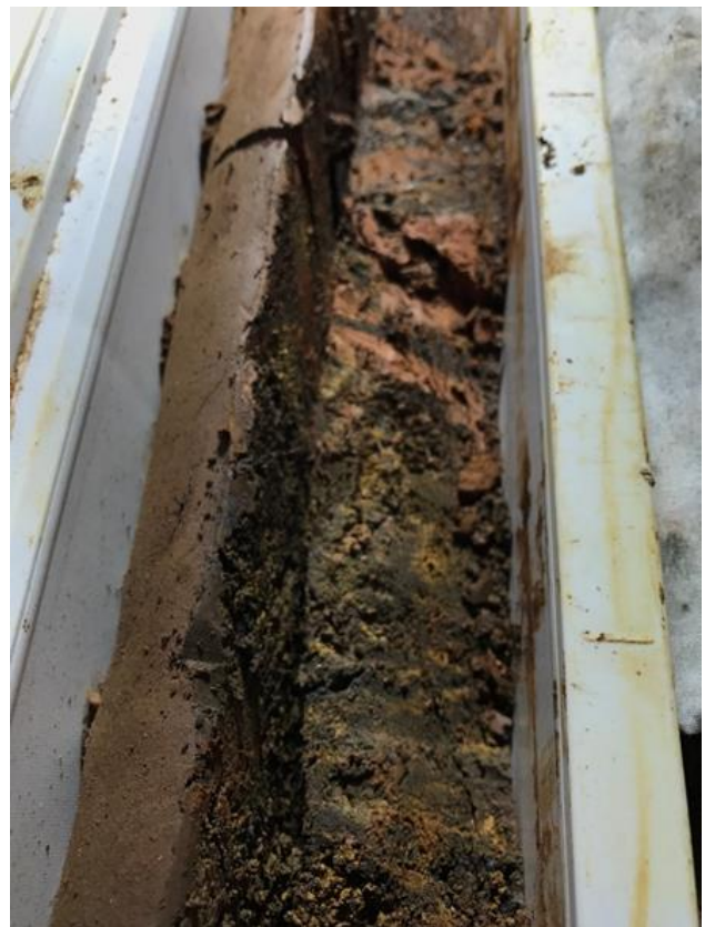
Figure 6 – High grade cobalt-nickel mineralisation from around 26.0 m depth in drill hole AGSD0004. As a rule of thumb, higher cobalt and nickel grades correspond to darker material in the drill core. The core in the centre of the left image contains strong mineralisation measuring 0.69 % cobalt and 2.07 % nickel.
