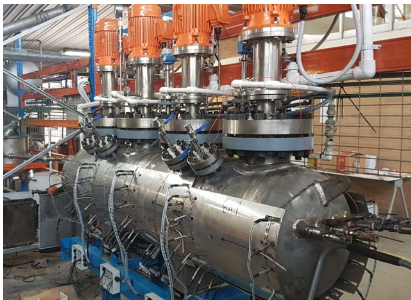
Figure 1: Pilot plant autoclave at Simulus ready for the Goongarrie bulk sample Research & Development
