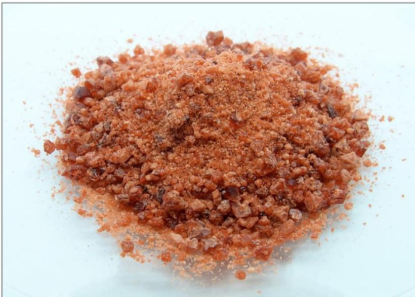
*Figure 3 - Cobalt Sulphate Crystals*
