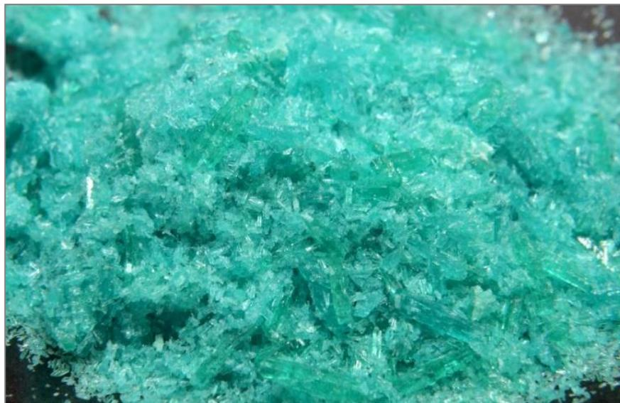
*Figure 1 –Nickel Sulphate Crystals*
