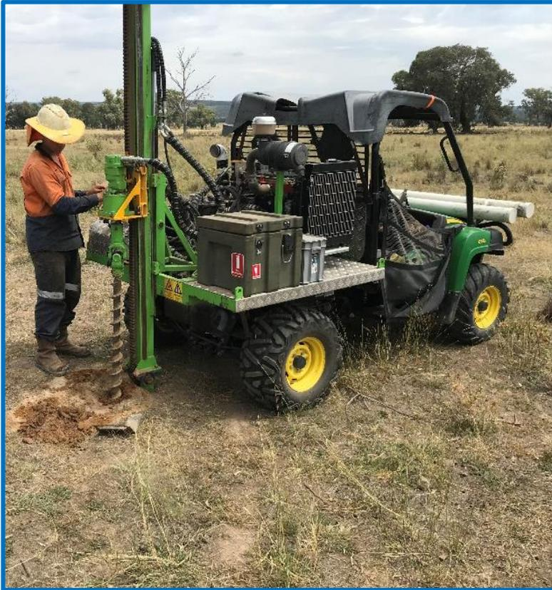
Figure 8: Soil auger sampling in progress.
