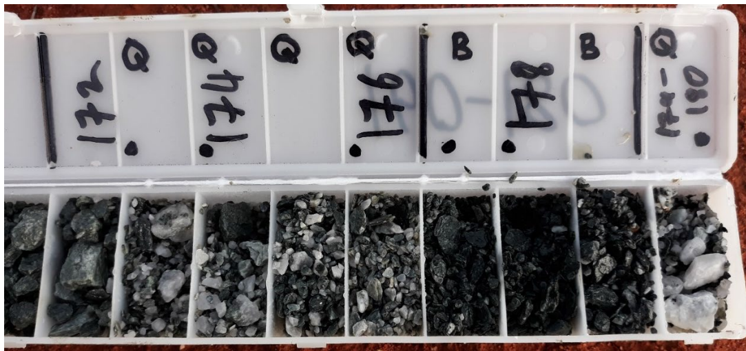
Figure 4 - Main Lode AANR0001, 172-180m End of Hole, 8m at 4.94g/t Au, altered dolerite with increasing foliation intensity, strong quartz-carbonate±sericite±biotite alteration and quartz-pyrite veining.
