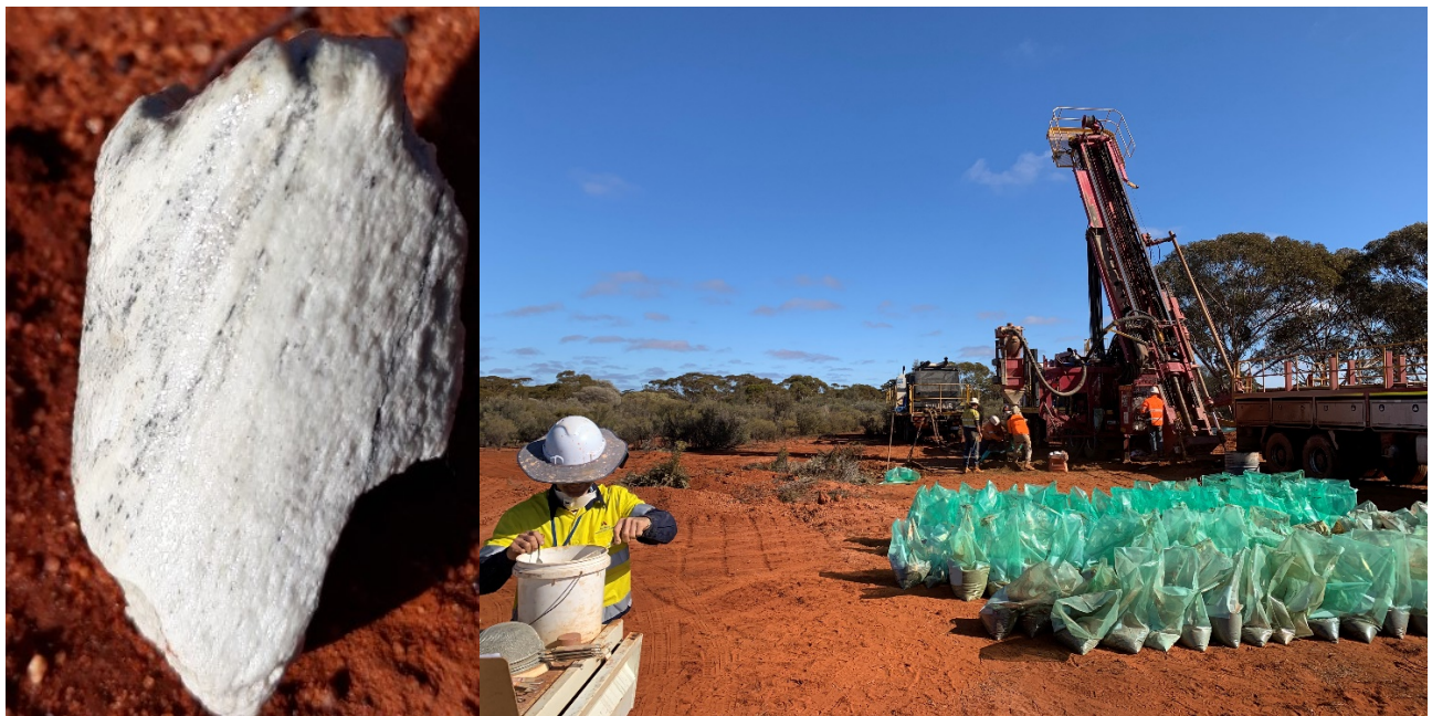
Figure 5 – Left: Core stick of strongly foliated, sericite and carbonate altered felsic volcanoclastic from aircore hole AGSA0033, supporting the interpreted steep dip shown in the geological interpretation in Figure 3. Right: RC drilling in progress at the first ever Aphrodite North RC hole, AANR0001. Looking west.
