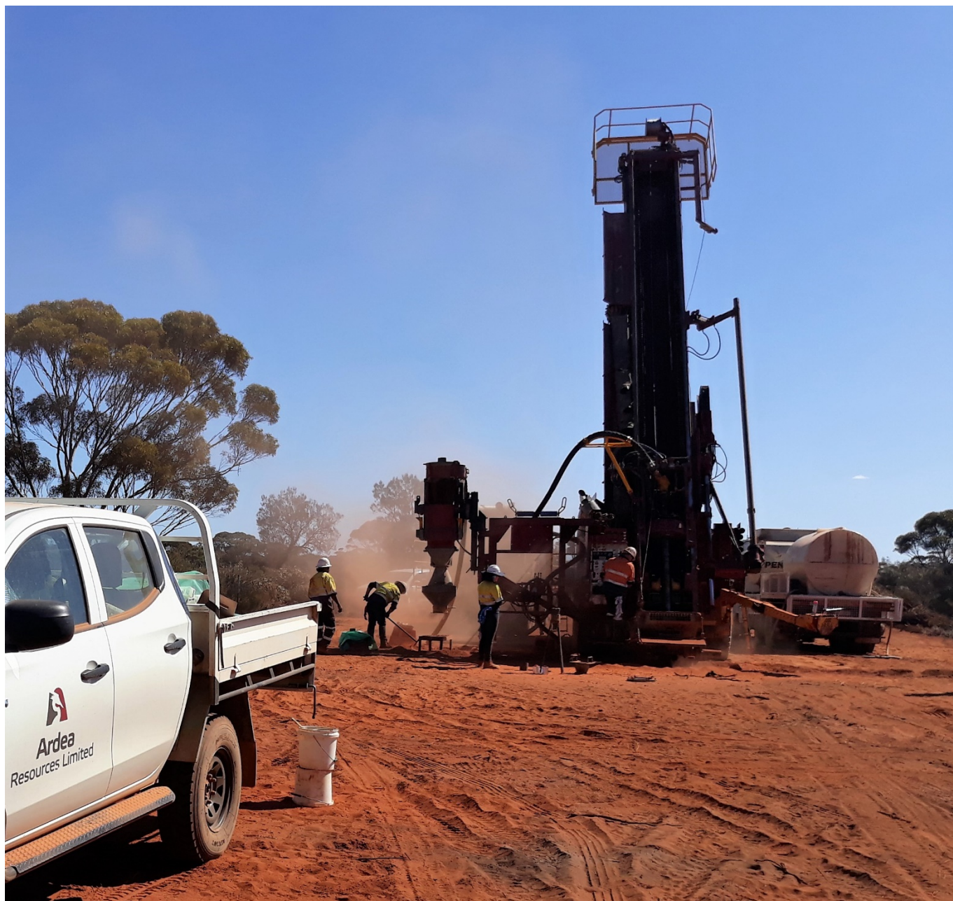
Figure 2 – RC drilling and logging in progress at Aphrodite North, 3km east of the GNCP nickel-cobalt resource.
