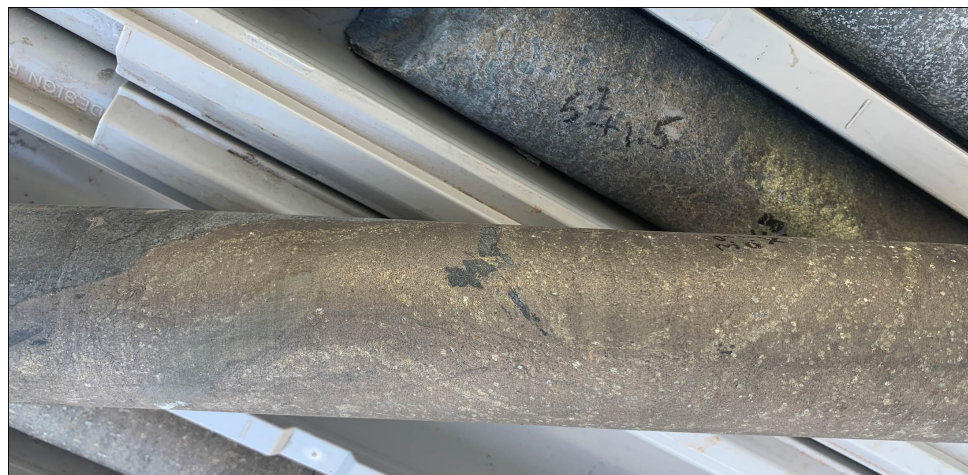
Figure 1: AELD0003, NQ2 core at 392.1m showing massive sulphide zone containing visible pentlandite (nickel sulphide), chalcopyrite (copper sulphide) and pyrrhotite-pyrite (iron sulphides).
