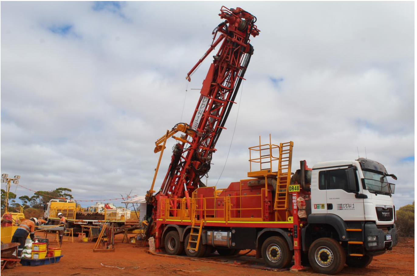
Figure 3: Diamond drill rig from industry-leading contractor DDH1 set up for drill hole AELD0004 at Binti South.
