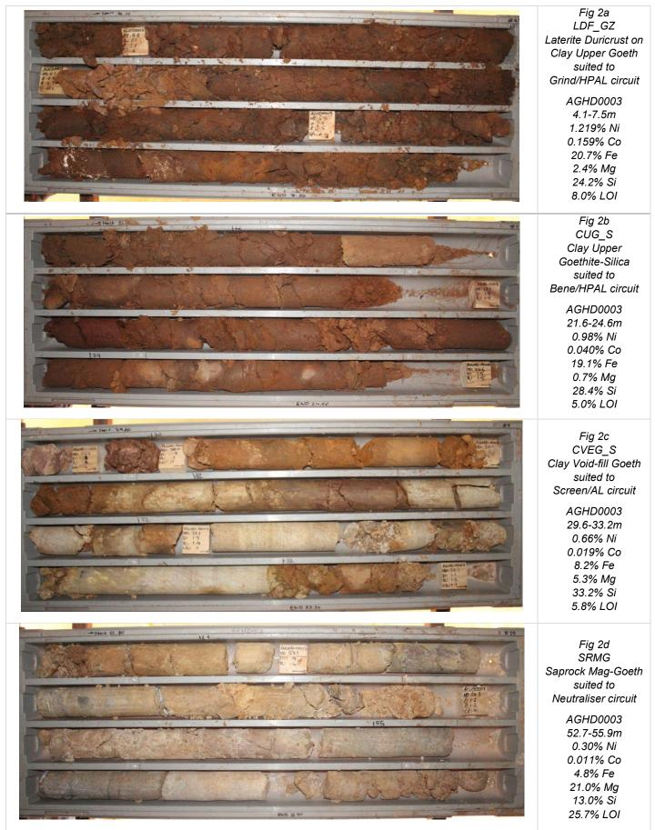
Figure 2: Goongarrie Hill Material Types, being a depth "pseudo-section" from Clay Upper, then Clay Void-fill, then Saprock being a typical laterite residual regolith sequence. The regolith code is first alphas for matrix, after "\_" for clasts.
