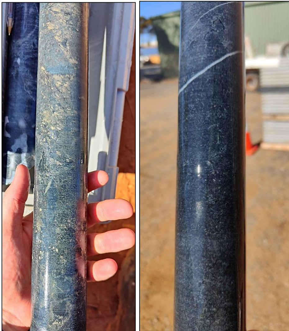
Figure 4: Left: matrix sulphides in AELD0008 (511.86m). Right: AELD0010 ultramafic with fine disseminated sulphides (132m)
