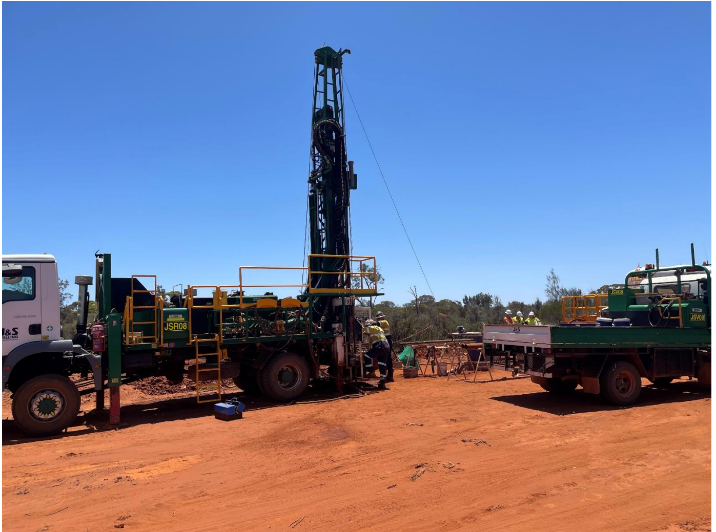
Figure 1: Diamond drill rig completing an RC twin hole for Quality Assurance and Quality Control assessment, as part of the Mineral Resource Estimate update that will be a key DFS deliverable.
