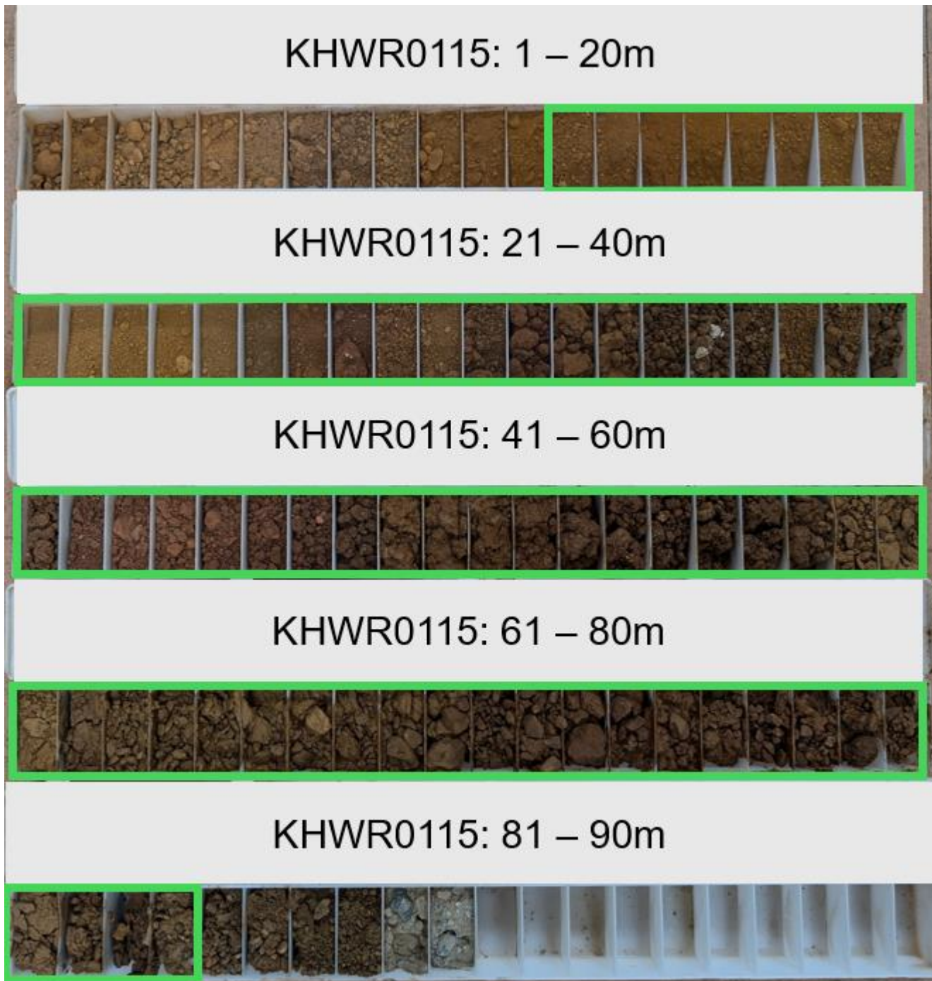
Figure 4 – KHW R0115 RC chip trays with significant intercept highlighted (72m at 0.92% Ni, 0.06% Co and 22.7ppm Sc, from 12m downhole)
