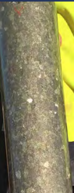
Massive Ni-Cu sulphides, Investigators prospect, drill hole MAD60, 5.3m @ 4.95% Ni, 2.75% Cu, 0.16% Co, & 5.25g/t PGE from 159.38m (St George Mining Ltd)*
