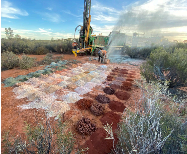
Aircore rig drilling at Ardea's GNCP, testing a gold geophysical target.
