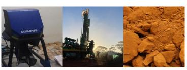
Ore Preparation testwork on Goongarrie was conducted at the Bureau Veritas laboratories. Spot analyses using a hand-held XRF enabled rapid, costeffective decisions to be made (Image used with permission of BV and RCS Australia).
