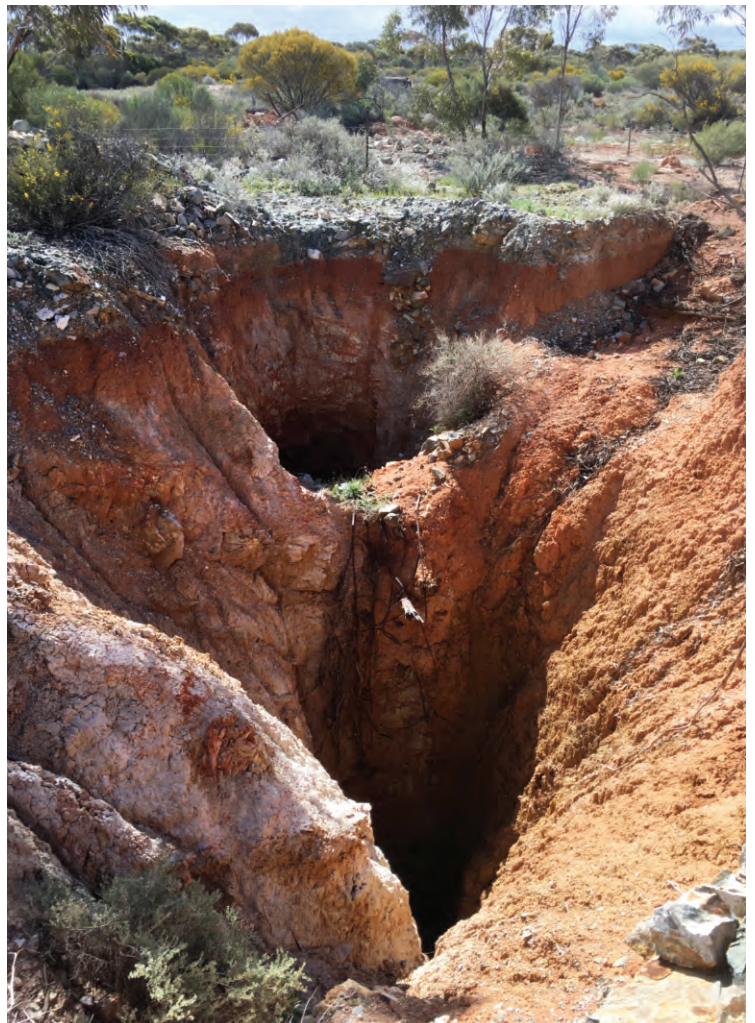
Facing north along the line of lode, collapsed stopes on old Big Four gold workings, note the sub-vertical massive white quartz reef in the lower left of photograph, hosted by yellow-brown clay altered diorite
