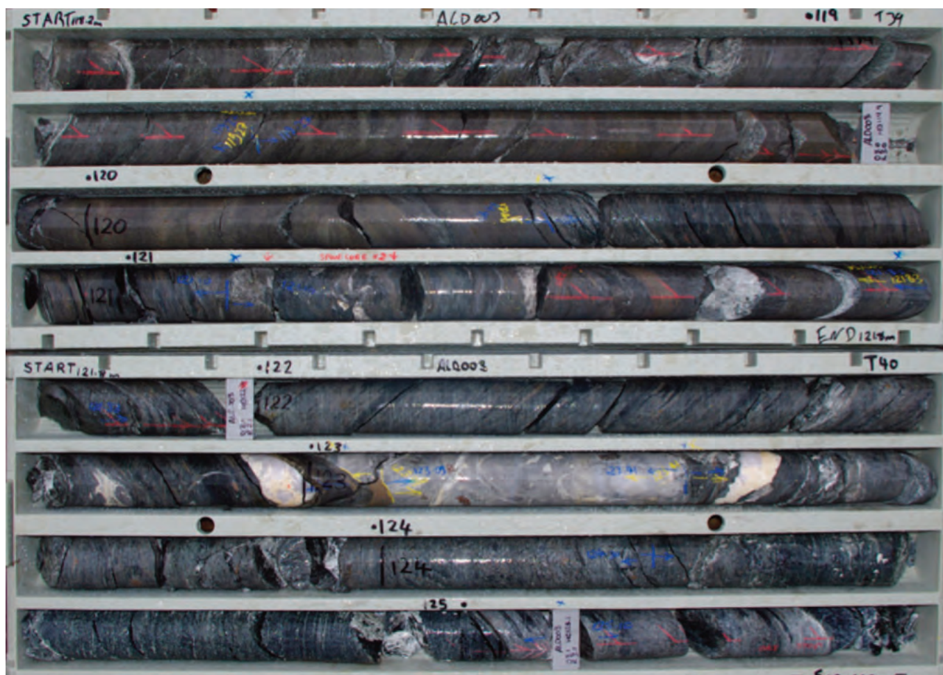
Figure 15 – Mineralisation in ALD0003 (119.27-120.48m, 1.21m at 14.29% Zn equiv), typical intense chlorite-pyrite alteration associated with Stringer Zone mineralisation
