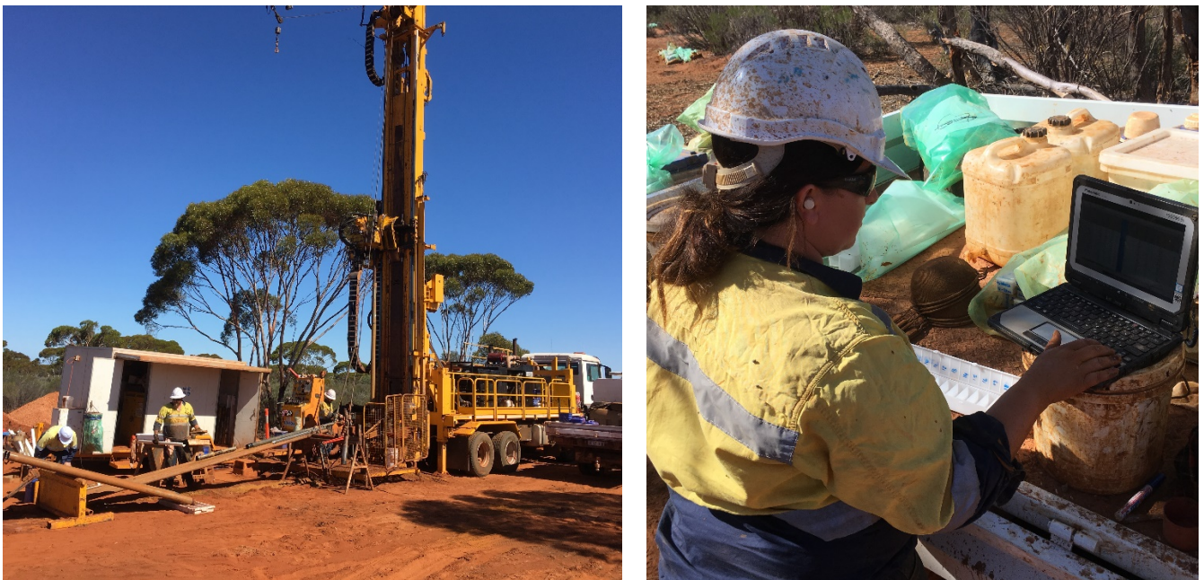
Figure 3 – Diamond rig Big Four, facing south, core for metallurgical variability program at Simulus (left). RC drill chip logging underway at the RC drill rig, Elsie North drill out and bulk sampling (right)
