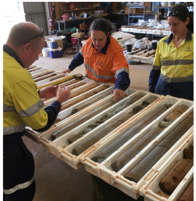
Figure 9 – Core processing facility, Ardea West Kalgoorlie office. The geological team examines drill hole AGSD0022 and selects drill core samples for Stimulus Engineering piloting bulk samples. The other racks are taken up by hole AGSD0015 which contains almost 100m of mineralisation, well suited to producing marketing sulphate samples
