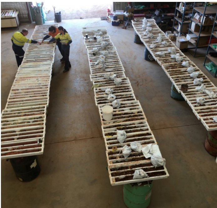
Figure 9 – Core processing facility, Ardea West Kalgoorlie office. The geological team examines drill hole AGSD0022 and selects drill core samples for Stimulus Engineering piloting bulk samples. The other racks are taken up by hole AGSD0015 which contains almost 100m of mineralisation, well suited to producing marketing sulphate samples
