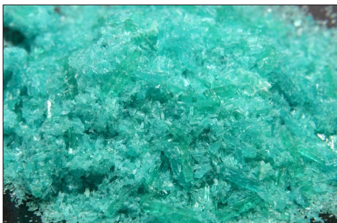
Photographs – upper red-orange cobalt sulphate, lower blue-green nickel sulphate produced from Goongarrie ore.
