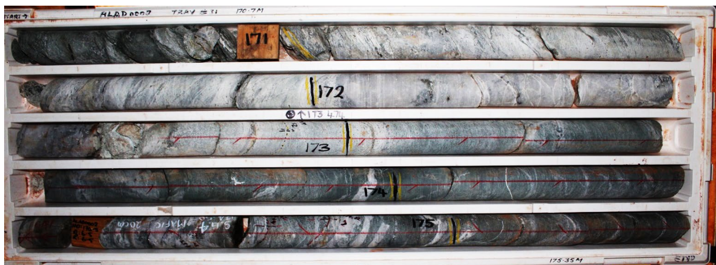
Figure 14 : Part of the main mineralised zone showing strong alteration and shearing of dolerite, with intense quartz-sericite-pyrite-chalcopyrite alteration evident 170.9–172.05m and 172.65–173.1m. Between these, there is a thick quartz(-pyrite-tourmaline-chalcopyrite) vein. Pervasive alteration is present up and down hole from this central zone. (ALAD0002, tray #31, 170.7 – 175.35m).
