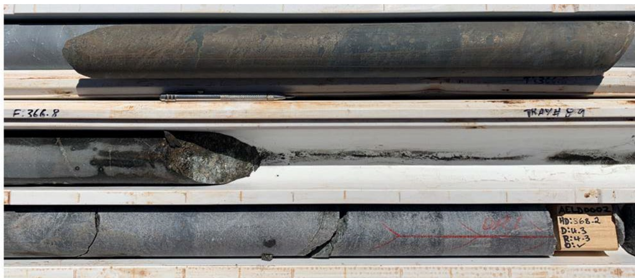
Figure 6: Recently completed Ardea diamond drill hole, AELD0002 showing massive (top) and disseminated (bottom) sulphides.
