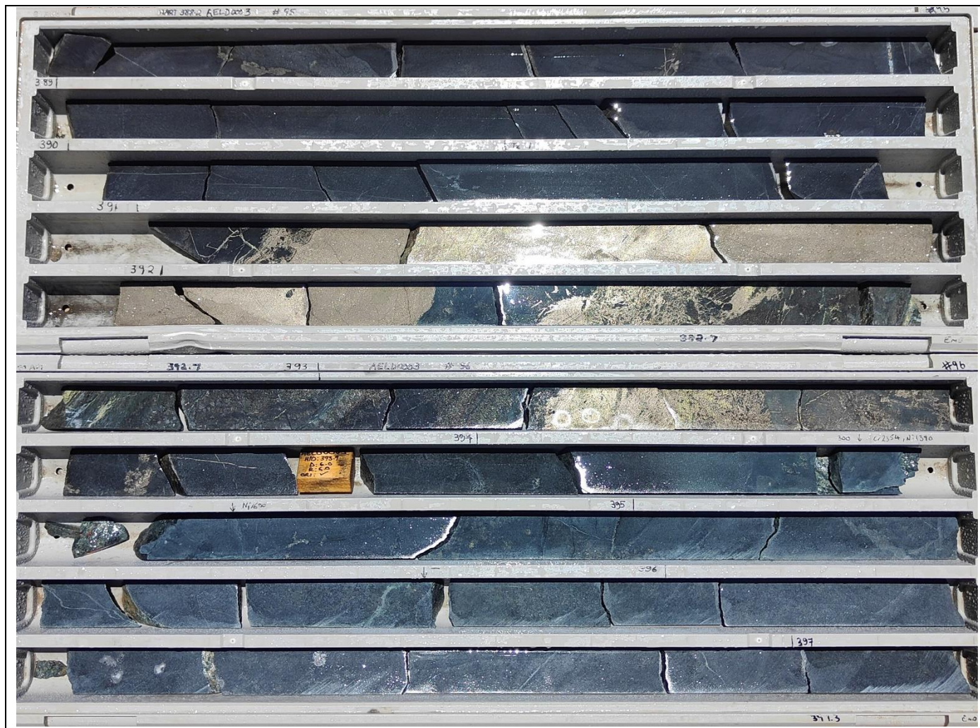
Figure 10: AELD0003, NQ2 drill core showing massive sulphide zone (391.04 – 393.76) and adjacent zones which exhibit high competency (solid core) and high recoveries. The core competency and lack of talc-chlorite shearing augurs well for good mining ground conditions. Note the down hole depth metre marks shown in black on the core trays.
