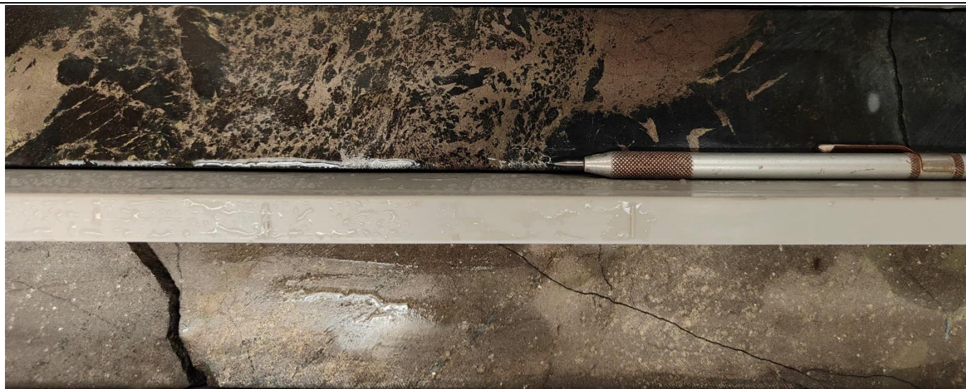
Figure 11: AELD0003 NQ2 drill core showing thermal erosion of the footwall dacite unit in the top section of the photo and massive nickel sulphide in the bottom section of the image.
