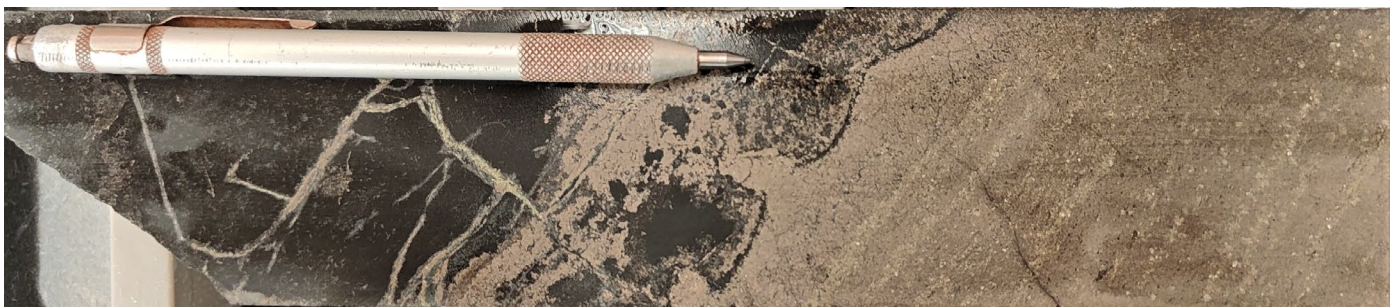
Figure 11: AELD0003, NQ2 drill core from 391.04m showing the dacite footwall contact and thermal erosion on the left-hand side of the photo and high-grade massive nickel sulphide on the right-hand side of the image.
