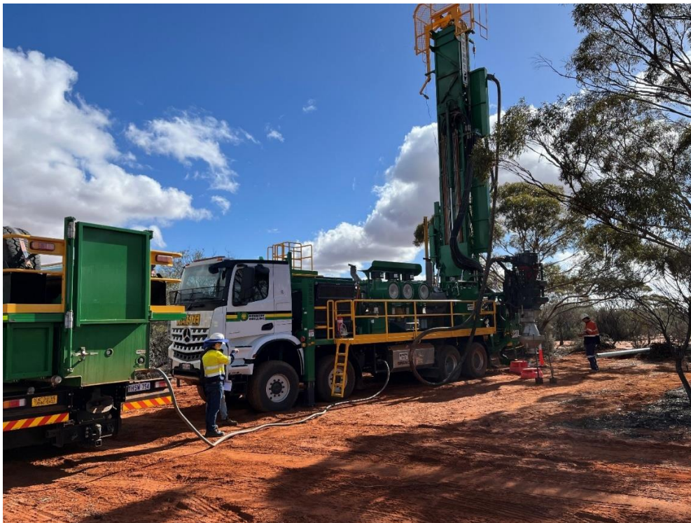
Figure 4: Infill resource definition drilling underway at the Big Four nickel-cobalt deposit, Kennedy Drilling rig.
