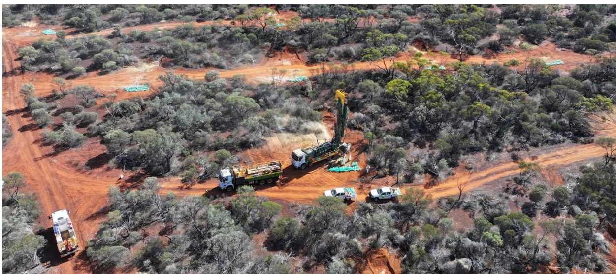
Figure 6: Infill resource definition RC drilling underway at the Goongarrie Hub.
