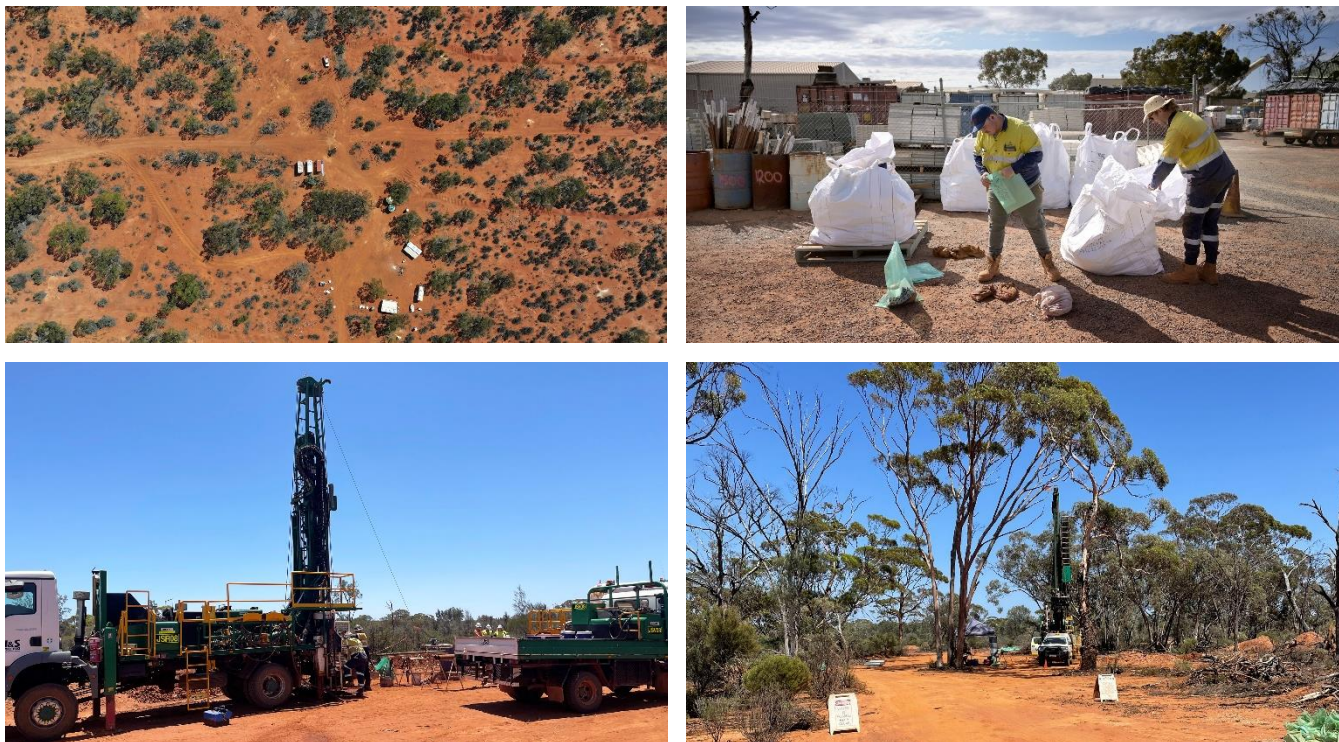
Figure 7: Top left: Goongarrie Hub Driller Camp; Top right: Sampling of RC drilling for assay submission; Bottom: Diamond core drilling underway.
